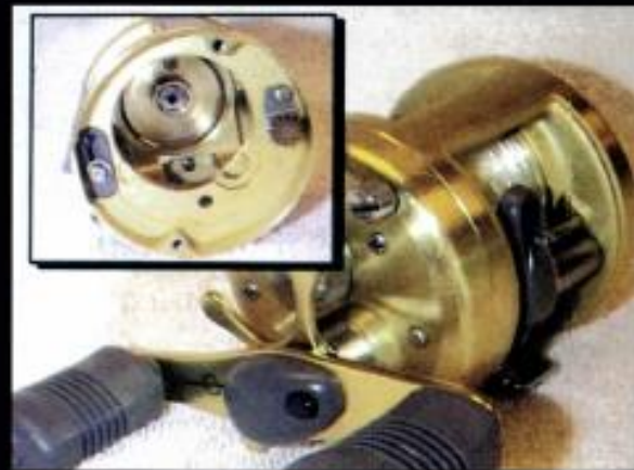
This six-year-old Shimano CT 250, used in saltwater and treated regularly with CorrosionX, shows no sign of corrosion inside or out.
